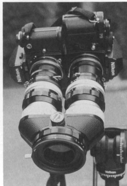
*"Milk Drop" was shot using a Stitz beam splitter stereo attachment in reverse on two Nikon F3s, with 105mm lenses and extension tubes in between. This provided a base of about 18mm. While the film planes were about 500mm from the subject, the "front" of the Stitz was only about half that distance. A full explanation of Mr. Flocks' sound trigger technique and examples of his high speed stereo work appear in color in the July/Aug. '92 Stereo World.*
